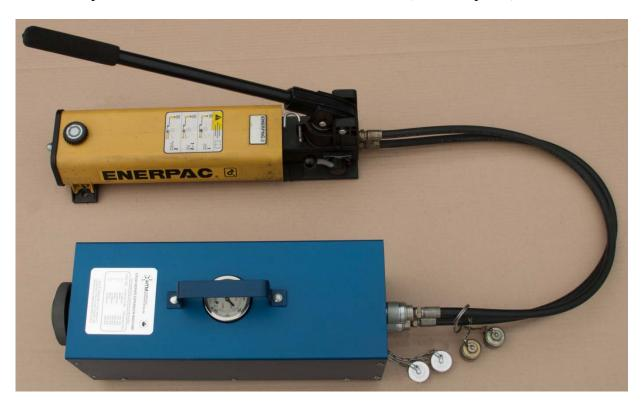
Connect Hose A to the lower quick-connect coupling. Connect Hose B to the upper quick-connect coupling.
