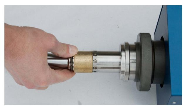
• Push the hose fully into the coupling, so that the hose contacts the coupling tail gasket squarely.
