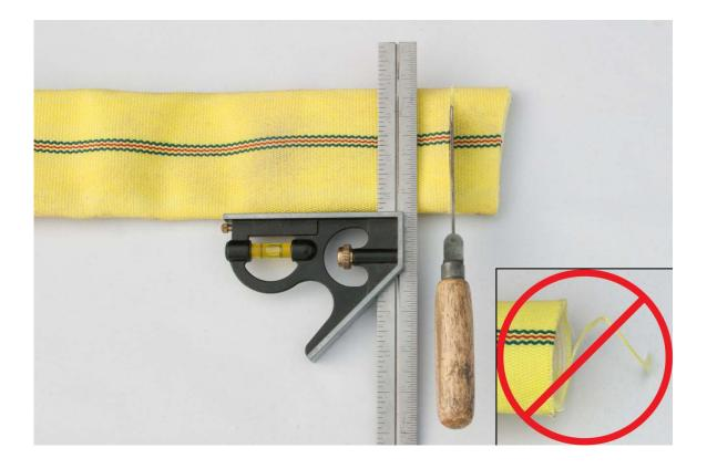
❖ The hose must be pushed all the way into the coupling, so that it contacts the tail gasket in the coupling.
