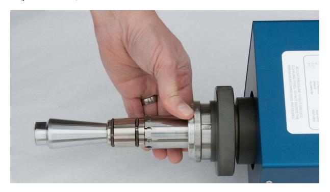
❖ Place the 1½" (Ø38mm) brass expansion ring over the CT150 expansion segments, exactly as shown in the photo.
