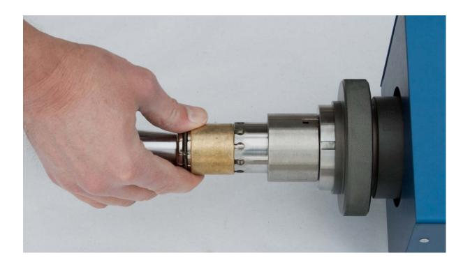
❖ Ensure that the Hose Coupling is properly positioned over the Expansion Segments of the CT150 Expansion Unit. Some couplings may require the use of a longer or shorter version of the CT1006 Adapter Sleeve.
