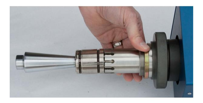
Tighten the adjustment wheel against the back spacer. This will maintain the correct depth of the expansion ring inside the hose coupling.
