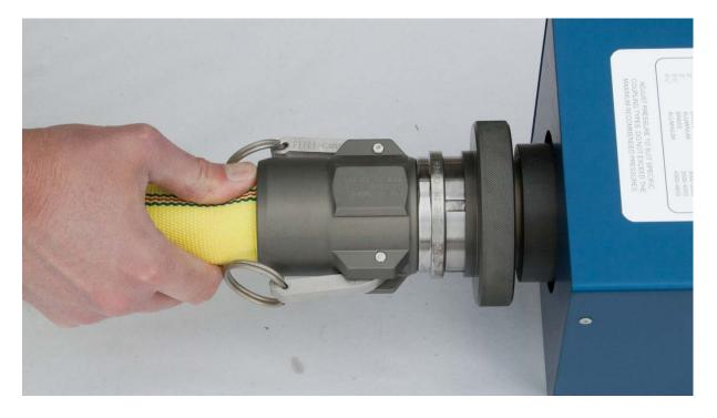
❖ Using the hydraulic pump with the valve in the "A" position, expand the ring to the recommended pressure.
